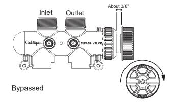
To return to SERVICE, turn the blue knob counter-clockwise (see directional arrow on end of knob) until the knob stops as shown.
